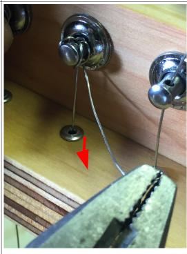
Swing the pliers to the right and up to the top. Once again, pull firmly to keep the wire neat against the peg and use your other hand to support the stub.
