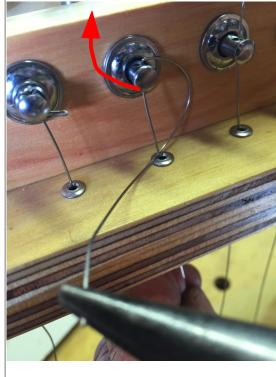
Using the pliers and while keeping a little pressure on the wire the whole time, swing the pliers towards you and down under the stub of the peg, and continue to take the pliers up to the right. The pliers should end up in the position shown here. You should find the wire has made a half-loop around the central wire, near the bottom of the hole.
