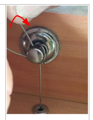
Grab it with pliers at the bottom, pull firmly as before, supporting the stub end with your other hand.
