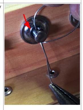
Use the pliers to pull the wire down quite firmly, while using your other hand to help guide the wire neatly around the curve of the peg. You want the wire to be tight around the peg and not falling off the end of the stub. You may also need to support the stub end of the peg while pulling firmly.
