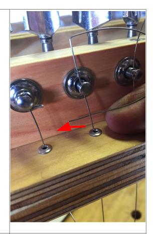
Pull the slack wire down with one hand so the right angle you made before is at the top of the hole. While doing this, grab the end of the wire with pliers, and lift straight up as shown in red. Pull firmly so the wire sits tight against the curve of the peg.
